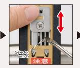
After operating the switch, put the holder plate back in its original position and securely tighten the screw.
