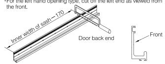
•If the distance between the cutting face of the rail and the reference mounting hole is no less than 120mm, make a new hole \$\phi\_5.5mm\$ at the position 50mm from the rail end.
