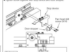
•Be sure to tighten screw, door stopper may come out of place. In case of the door open strongly, install the door stopper in
