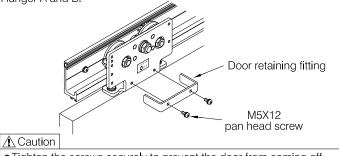
• Tighten the screws securely to prevent the door from coming off.
