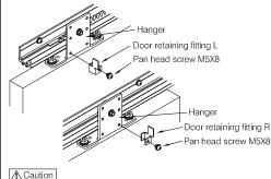
Be sure to install the door retaining fitting, the door may come
