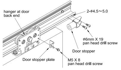
Tighten the screws securely to prevent the door from coming off.
