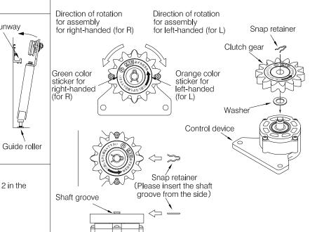
• When assembling and reengaging the clutch gear, be sure to turn it printed direction. If push roughly, the clutch gear may breakdown.
