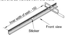
If the distance between the cutting face of the rail and the reference mounting hole is no less than 80mm, make a new hole \$\phi 5.5mm for installing the rail at the position 50mm from the end.
