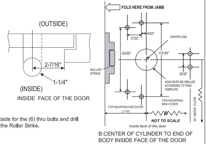
Drill 9/32" holes inside and 3/8" holes outside for the (6) thru bolts and drill & tap for (3) 1/4"x20 machine screws for the Roller Strike.
